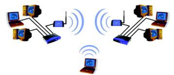
Figure 2-3: Wireless Bridging Using Two Bridges
